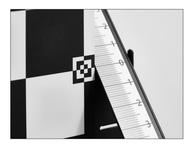
Attach your camera to a sturdy tripod. You want to make sure that your camera and SpyderLENSCAL are the same height. Adjust the height of your tripod and SpyderLENSCAL when they are next to each other. The center point on the vertical piece of the SpyderLENSCAL should be in the center of your lens when the camera is level. Using a light stand makes adjusting the SpyderLENSCAL to the height of the camera very simple.
