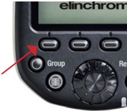
PWR Button(control Brightness of Neo 2)
