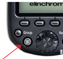
Test Flash Key (Single Click=right click, Double click=left click from Neo 2)
