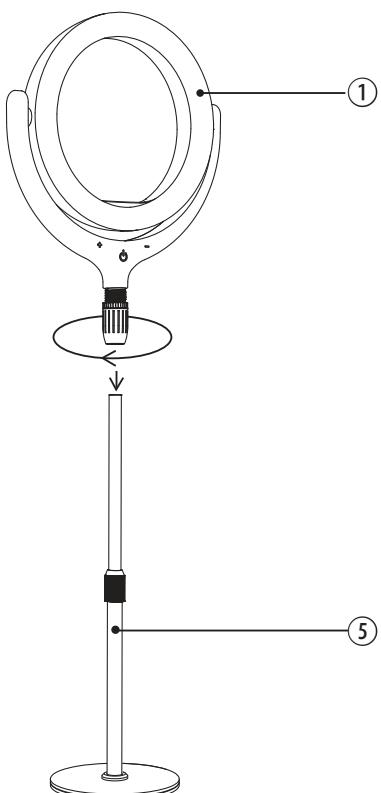
**Step 1** :Screw the stand (5) into the base plate (7).
