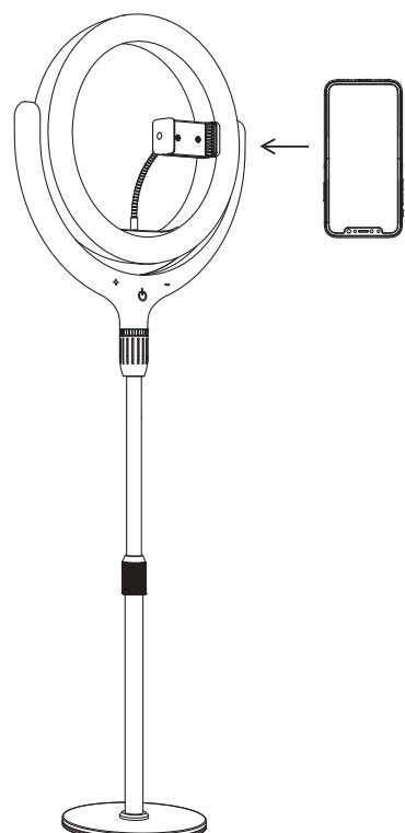
**Step 3:** Insert the flexible arm (2) into the ring light (1). Press the smartphone holder (10) into the ball joint of the flexible arm (2).
